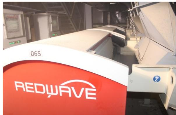
Picture: REDWAVE Sorting Machines for colour sorting and separation of contaminants
