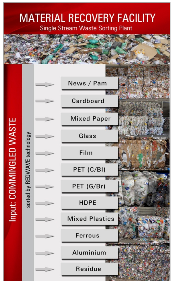
Infeed material is sorted in 12 different fractions
